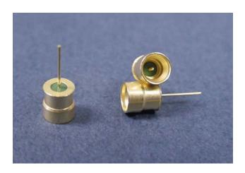
Our SMPM aluminum compatible RF connectors are manufactured to MIL-STD-348 with unique processes and controls to assure compliance with all specified properties. Particular attention has been given to plating control to assure required plating thickness. Minimum plating on pins is guaranteed for wire and ribbon bonding. Limited plating on housing is assured to prevent gold embrittlement when soldering with Sn and SnPb based solders and also to preserve dimensional precision.
